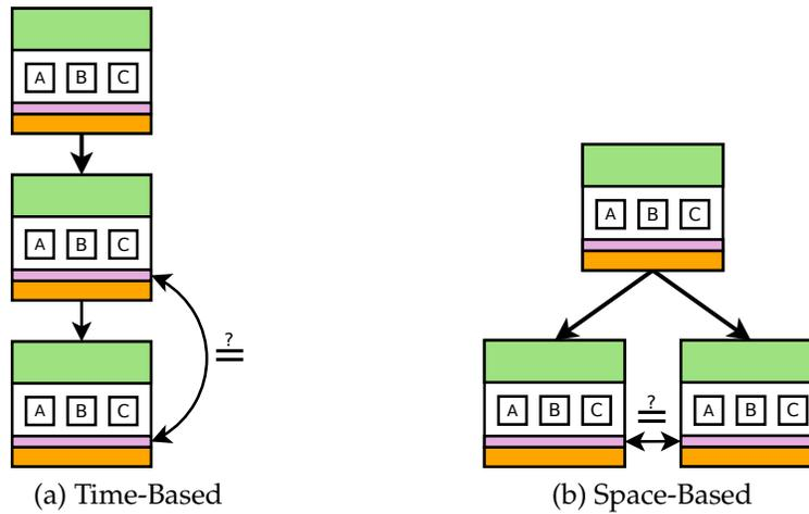
Figure 3: Two ways of providing periodic error detection with redundant Containment Domains. The outputs of each are compared at the end of execution; if an error is detected, a likely recovery mechanism would re-execute given fresh inputs from the parent.
