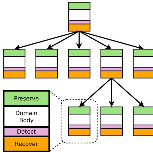
Figure 1: The organization of hierarchical Containment Domains. Each domain has four components, shown in color. The relative time spent in each component is not to scale.
