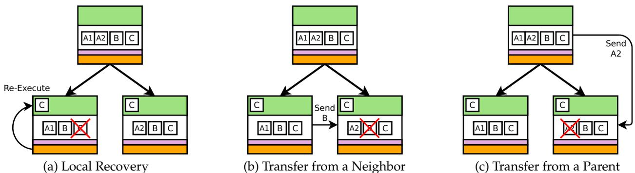
Figure 2: Examples of recovery after the detection of a failure in some input. Both local restoration (a) and optimized recovery through restoring data from non-local domains (b and c) are shown.
